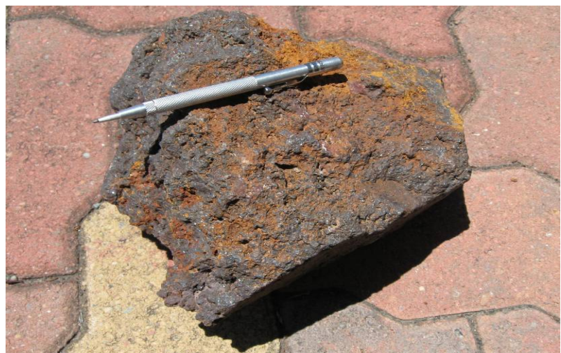
Figure 4: Ironstone from the Hicks Quarry assaying 67.8% Fe
