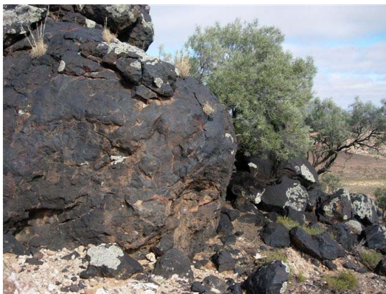
Figure 1: Massive magnetite/haematite outcrop assaying 65-67% Fe
